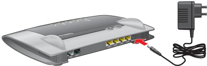
NOTE! After a few seconds the Power / DSL LED should start flashing. It means your FRITZ!Box is ready for operation. In case this LED doesn't flash and stays off, contact our customer service center on 03 265 67 00.
